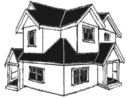
Effective use of separate entrances in a duplex provides for the appearance of a single family dwelling
