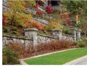
Figure 45. Stepped retaining walls help reduce visual disruption when compared to tall walls
