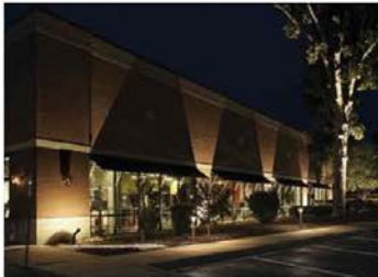
Figure 36. Down lighting with cutoff shields reduces glaring light sources.
