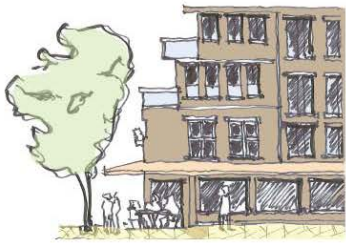
Figure 12. 2 storey street wall with upper storeys stepped back a minimum of 1.5m
